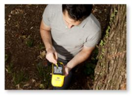
Trees and buildings create "satellite shadows", limiting the areas where you can reliably collect high-accuracy GNSS data. Using Trimble Floodlight technology, the GeoExplorer 6000 series continues to deliver productive, usable data under tree canopy or in urban canyons. You can work with fewer disruptions, meaning better data, faster, at less cost.
