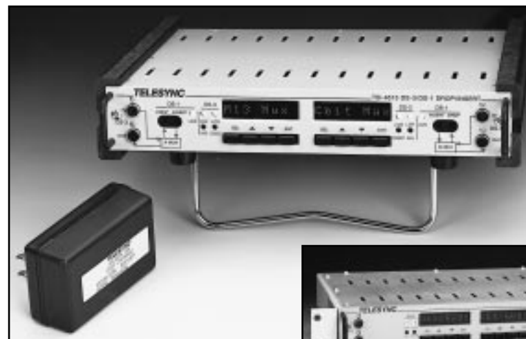
Model TSI-4515 in option-1 portable 110 VAC configuration. Portable configurations are available for all models.
