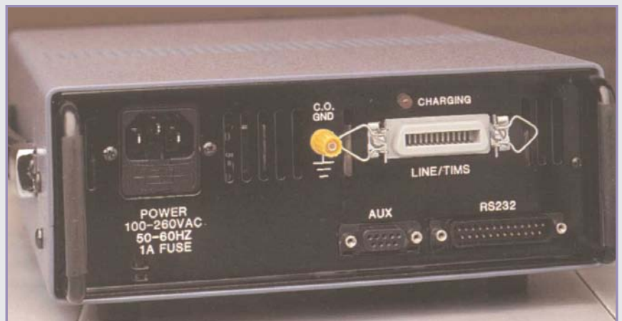
Rear of AM8a with RS232 ports for hard copy output and remote control.
