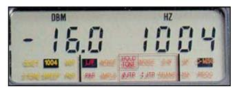
Large easily-read LCD with simultaneous display of test set-up menu and measurement.
