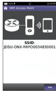
OneExpert providing WiFi access point
