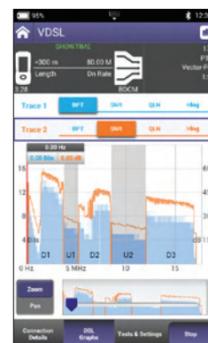
Bits-per-tone (BPT) vs SNR graph
