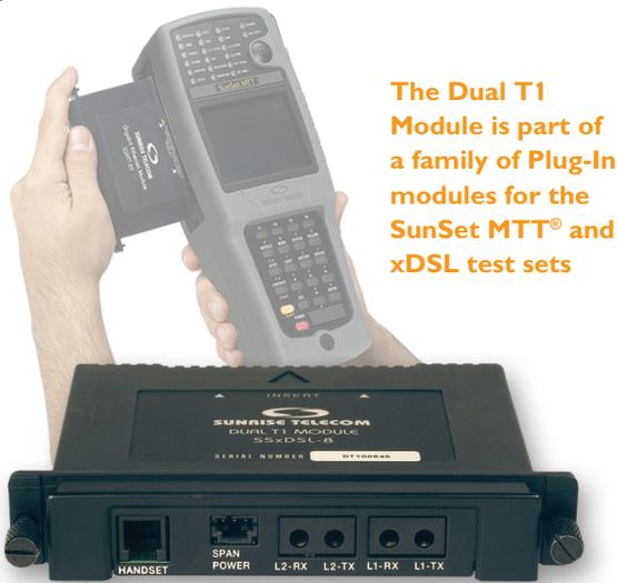
The Dual T1 Module is part of a family of Plug-In modules for the SunSet MTT® and xDSL test sets
