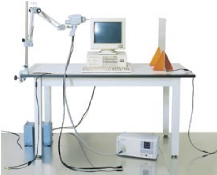
Test set-up example with ESS-801
