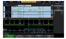
Figure 19. Multi-bus time aligned decode.
