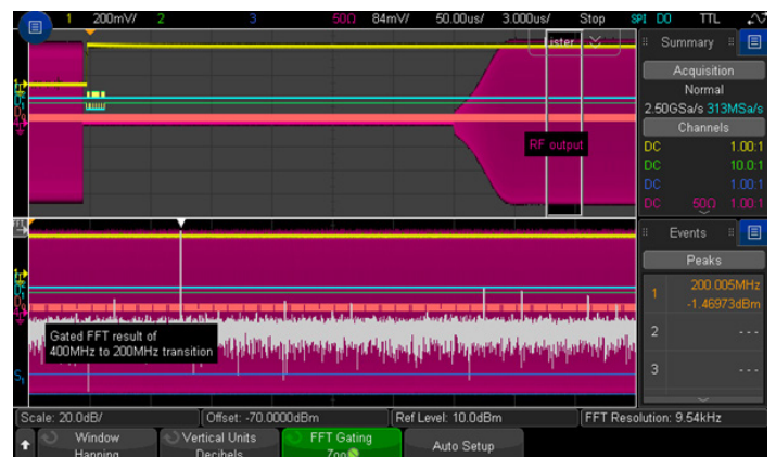
Figure 21d. RF signal settled down at 200 MHz as indicated in the search lister.
