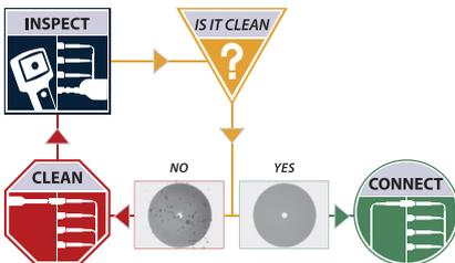
**Contamination is the number 1 reason for troubleshooting optical networks.** Proactive inspection and cleaning of fiber connectors can prevent poor signal performance, equipment damage, and network downtime.
