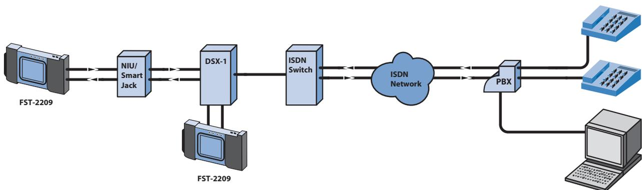
Verify or troubleshoot your customer's ISDN PRI service using the FST-2209 module's ISDN testing capabilities
