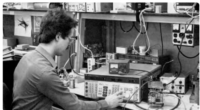
The 8663A's low noise and high output power are ideal for local oscillator substitution applications.
