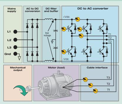
In three-phase systems like variable speed drives, UPS or back-up generators, use four channels to diagnose power input, dc to ac converters, or cable interface problems.
