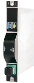
FTBx-740C-CWDM or FTBx-740C-DWC single module for FTB-1v2 single- and dual-carrier FTB-2/FTB-4 Pro mainframe
