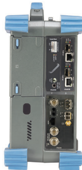
The FTB-8510G Packet Blazer 10 Gigabit Ethernet Test Module is housed in the FTB-400 Universal Test System, EXFO's rugged, all-in-one portable platform. Also shown in the platform, the FTB-8510B Packet Blazer Ethernet Test Module and the FTB-8120/8130 Transport Blazer Next-Gen SONET/SDH Test Module.
