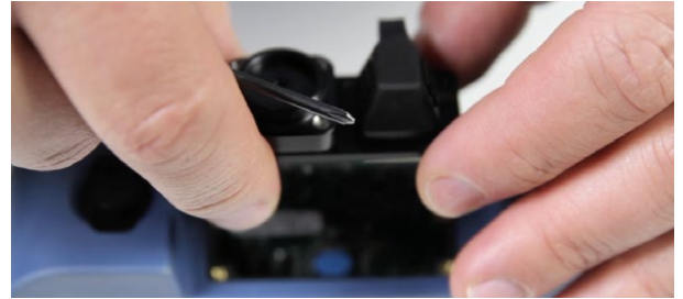
The easy-to-install power meter and VFL pieces attach to the MAX-FIP display using four screws.
