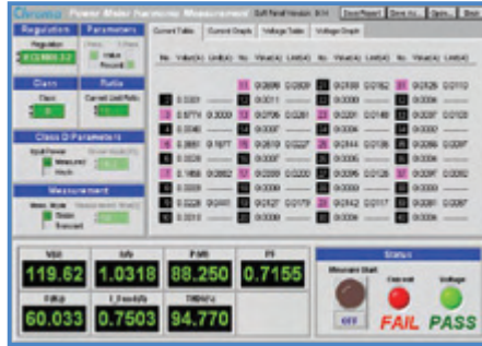
IEC 61000-3-2 Current Harmonic Test
