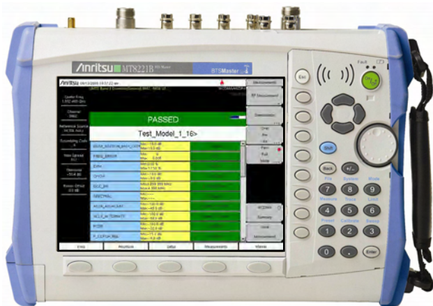
BTS Master in Pass/Fail Mode
