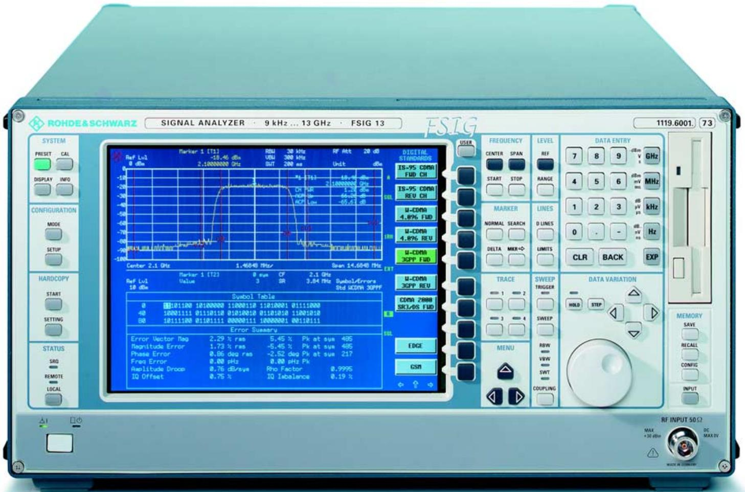
The RMS detector available for all bandwidths up to 10 MHz is the ideal tool for precise power measurements whatever the waveform. Channel power and adjacent-channel power can accurately be measured and displayed irrespective of any signal statistics. Measurement challenges like repeatability of power measurement of modulated signals (eg CDMA) can thus be eliminated.
