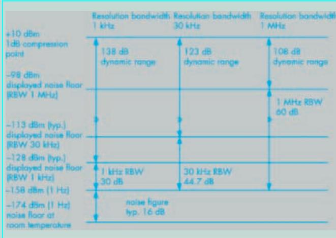
Dynamic range, noise, and 1 dB compression point of Signal Analyzer FSIG3
