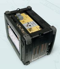
The powerful STT Optical Network Expert (ONE) module simplifies the complex tasks of installing and maintaining OTN networks. The STT ONE verifies a wide range of network performance issues, including end-to-end connectivity, forward error correction capabilities, asynchronous/synchronous mapping of SONET/SDH client signals, and conformance to ITU-T G.709 OTN recommendation.
