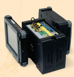
The STT Metro module combines Ethernet and Fibre Channel test and measurement capabilities in a single instrument.
