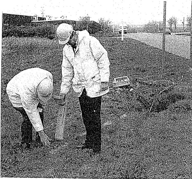
The RD400PXL is a Precision Locator comprising a receiver and a transmitter for pinpointing buried utility lines in congested and complex situations in the highway or on an industrial site.
