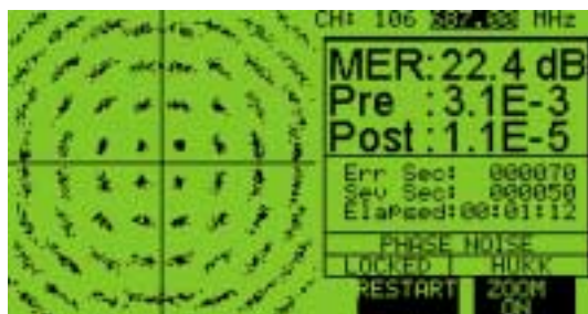
64 and 256 QAM Measurements with Hukk's exclusive Automatic Constellation Diagnosis.
