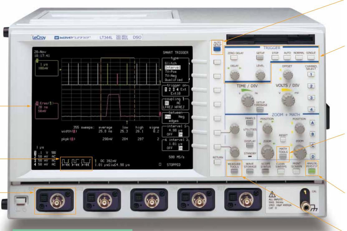
**Autosetup** adjusts the scope to automatically display the signal.
