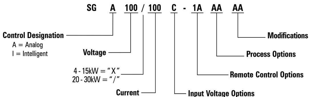
(For units up to 999A, Current is represented in numeric format (rounded to whole Amp), e.g., above "100" represents 100A. For units at 1000A and above, the current is represented by the format "XKX", e.g, 1K2 represents 1200A)
