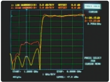
The Return Loss measurement of a low pass filter is grossly distorted when high harmonics are present. When the source's fundamental frequency passes 2 GHz, the second harmonic (at 4 GHz) enters the lowpass filter's reject band; thus, 100% of the second harmonic power is reflected back toward the source. Thus, the reflected harmonic power is measured and then erroneously displayed as the return loss characteristic between 2 and 4 GHz.
