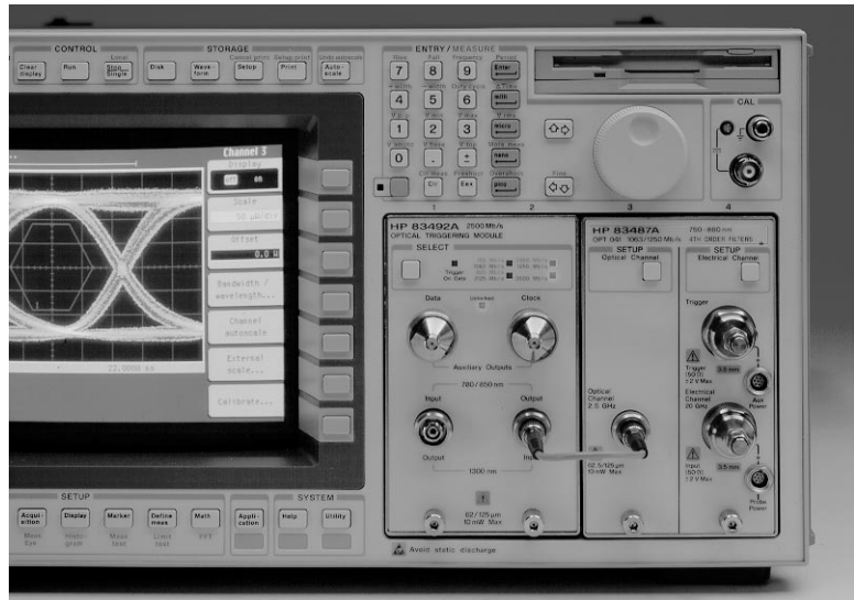
HP 83480A with the new HP 83492A Clock Recovery Module and HP 83487A Datacom Reference Receiver
