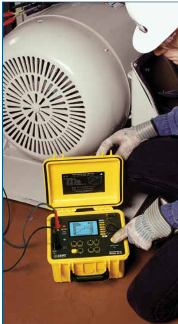
Model 5060 checking insulation resistance on feed cables to a three-phase motor.
