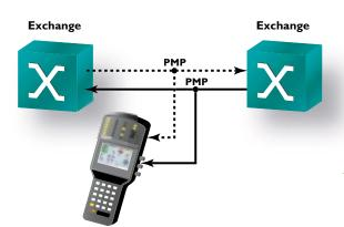
Long-term monitoring is simple with the SunSet E20c. Program a start and stop time, and the SunSet E20c takes care of the rest. The set may also be configured to print out every error or alarm condition, along with a date and timestamp. Histograms provide a graphical record of errors and alarms through time for easier correlation of repeating problems.
