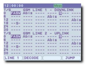
**TRAU Testing:** The SunSet E20c can insert an artificial voice message into a GSM subchannel to check voice conversion in the TRAU units. Full duplex testing means the SunSet E20c can insert a speech message or 16 kbit/s data pattern on an in-service link. C-bit manipulation can stress test the network's response.
