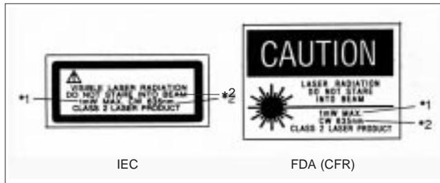
The maximum output is indicated under \*1, and the wavelength under \*2. Caution: Do not look directly into the laser beam.
