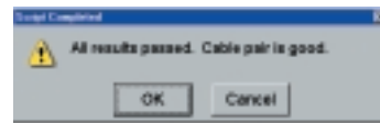
The Good Pair Check returns either a pass, marginal, or failed result to remove the guesswork from testing.
