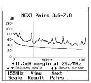
Detailed NEXT results screen shows the measured data as well as the pass/fail limit curve defined by the selected test standard.
