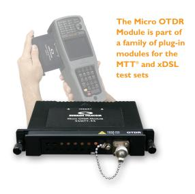
The MTT-35E Micro OTDR Module, part of the Modular Test Toolkit (MTT) family of products, is a rugged, battery-operated handheld test solution for the installation and maintenance of fiber optic cable. The Micro OTDR module is the first in its class to provide an optical time domain reflectometer in a compact module that measures fiber optic cables for events such as connectors, splices, breaks, and insertion loss.
