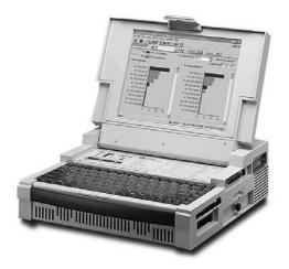
The auroraDuet troubleshooting capabilities provide testing of local loop at the U-interface, in TE mode it simulates terminal equipment and validates line operation on S/T and U interfaces, checks cable continuity to S bus problems, and monitors D-Channel traffic on S/T and U interfaces for problem analysis.
