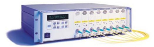
79710 Fiber Optic Switch Module is designed and optimized for high return loss, low insertion loss and excellent stability. This optically passive fiber optic switch is transparent to signal formats and bandwidths as well as being bi-directional in operation. A choice of timed, random, sequential or triggered switching modes enhances switch module functionality.
