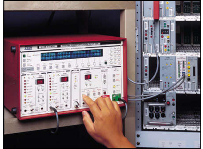
The 440B/T-ACE is a multi-purpose digital communications analyzer, ideal for Central Office and CPE testing.
