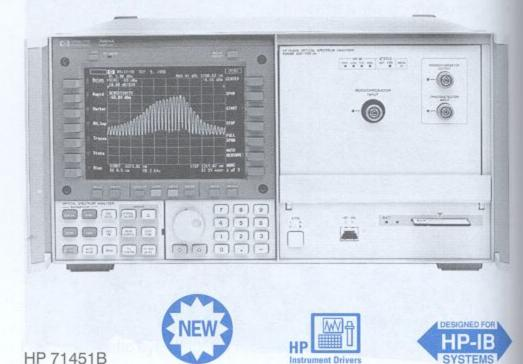
An optional white light source covering 900 to 1600 nm can be added to your OSA for swept wavelength stimulus response testing of optical components. The optical spectrum is filtered below 900 nm to prevent errors due to detection of light at half the wavelength of interest.
