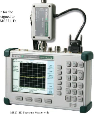
MS2711D Spectrum Master with FCN4760 block down converter
