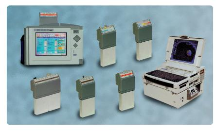
All Agilent test modules, including the TDR Module, can be used interchangeably with both Agilent's Service Advisor portable test tablet and Internet Advisor PC platforms. Modules plug directly into the Service Advisor tablet or Agilent's Service Advisor Undercradle, which attaches to the Internet Advisor network analyzer.
