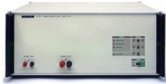
The 5220A Transconductance Amplifier lets you calibrate alternating or direct current meters and shunts and the current functions of digital multimeters that measure up to 20A. A known input voltage of 1 to 20 volts produces a known output current of 1 to 20A.
