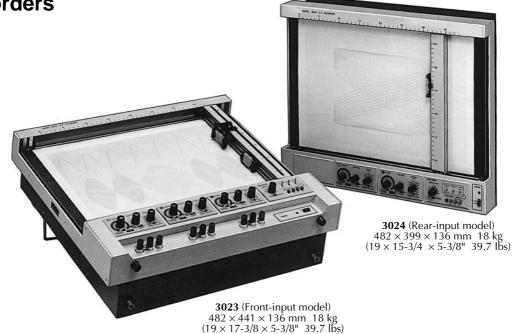
The 3023 and 3024 are top-level, high performance A3 X-Y recorders, available in front- or rear-input models, and one-or two-pen models. All models offer the fastest slewing speed and acceleration. The slewing speed and acceleration of the one-pen model in the Y axis is 2,200 mm/s 7.6 G, and 2,000 mm/s 5.1 G in the X axis.
